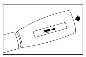
Your vehicle is equipped with a tow/haul mode. The button is located on the end of the column shift lever. You can use this feature to assist when towing or hauling a heavy load. See "Tow/Haul Mode" under *Towing a Trailer on page 4-62* for more information.
